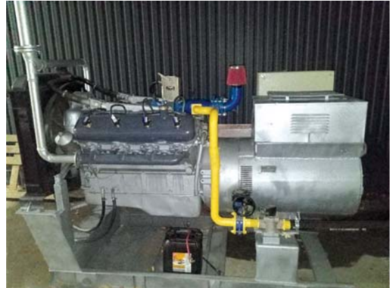
Open-frame gas engine power plant. Fuel: producer gas
