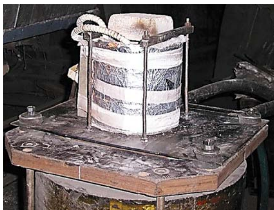
Laboratory furnace with electromagnetic stirrer for preparing master alloys
