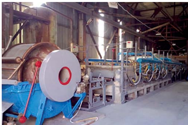
Continuous line for basalt insulation cardboard production
