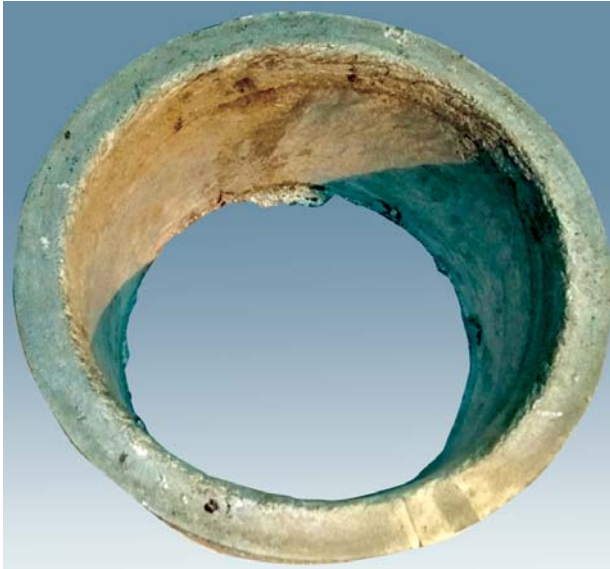
Aluminum alloy castings with diameters of 400 mm (left) and 150 mm (right), produced by centrifugal casting
