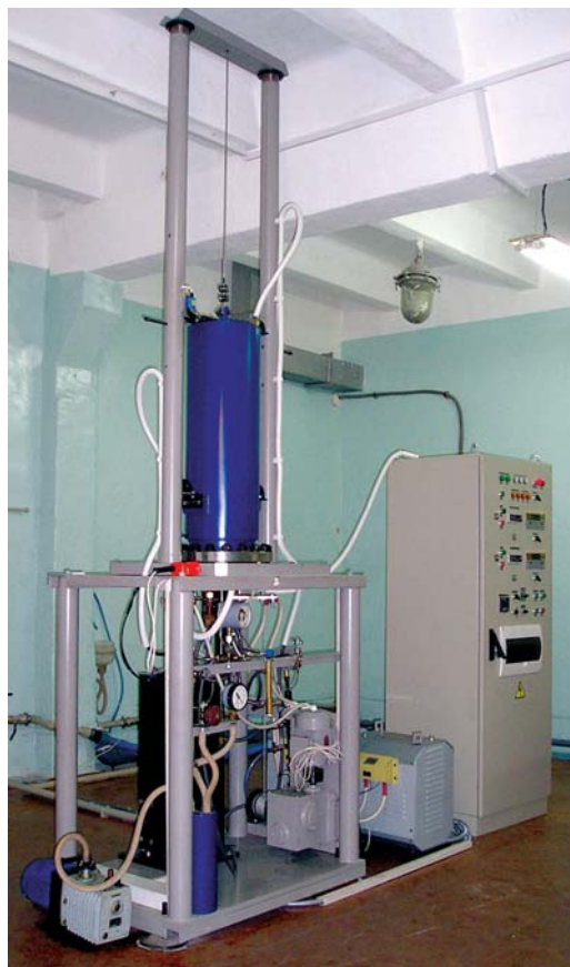
Equipment for growing A II B VI chalcogenide crystals using the vertical Bridgman method, under excessive inert gas pressure
