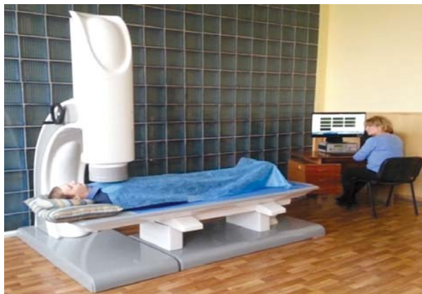
SQUID sensor magnetometric system (one of the options)
