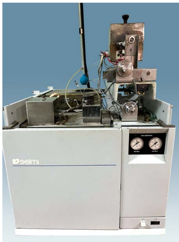
Installation for precision analysis of hydrogen in metals and alloys
