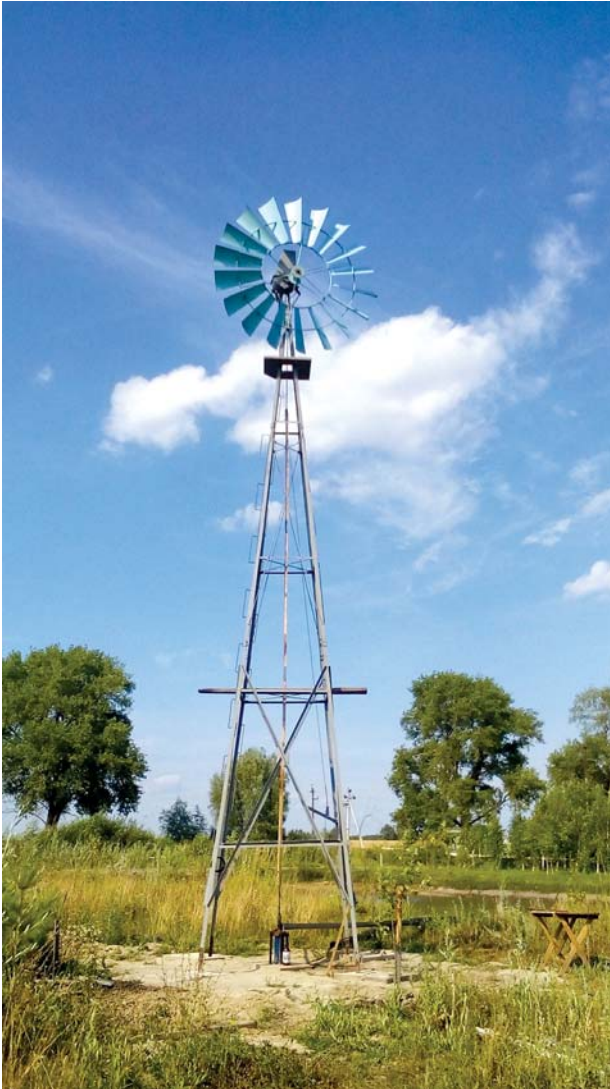
Prototype of a wind pump (Polubotky Village, Chernihiv region)
