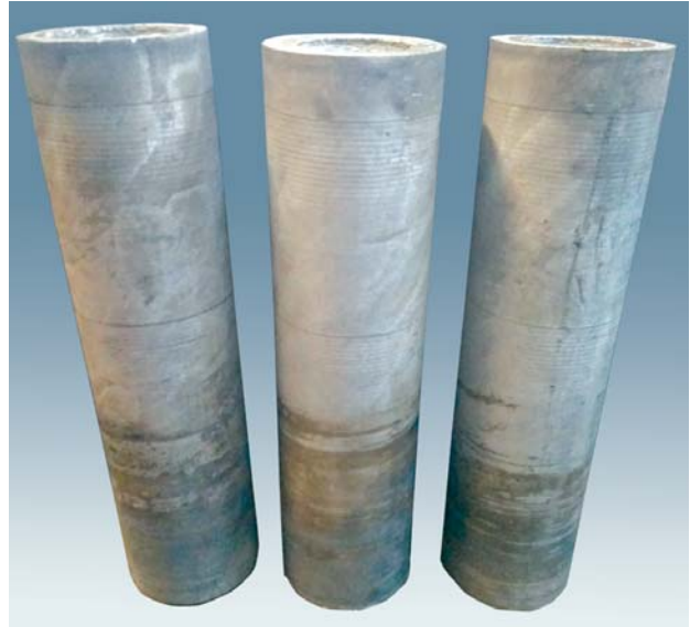
Aluminum alloy castings with diameters of 400 mm (left) and 150 mm (right), produced by centrifugal casting
