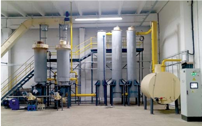
Gas generator set with generator gas purification system
