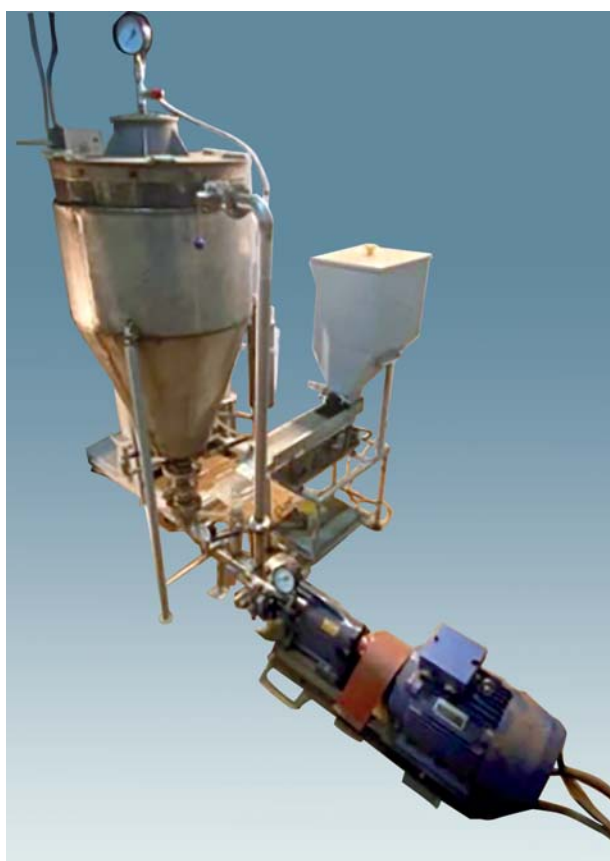
Installation for the production of bioethanol from lignocellulosic raw materials
