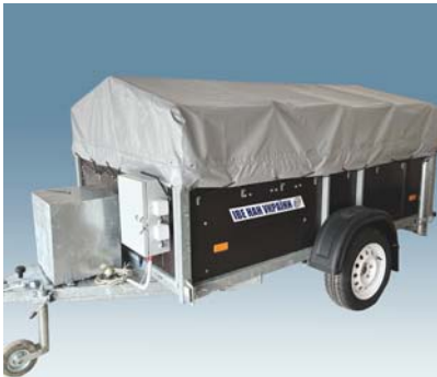
Mobile autonomous power supply system based on a car trailer: in transport mode (left), deployed mode (center), and deployed mode – side view of the trailer (right)
