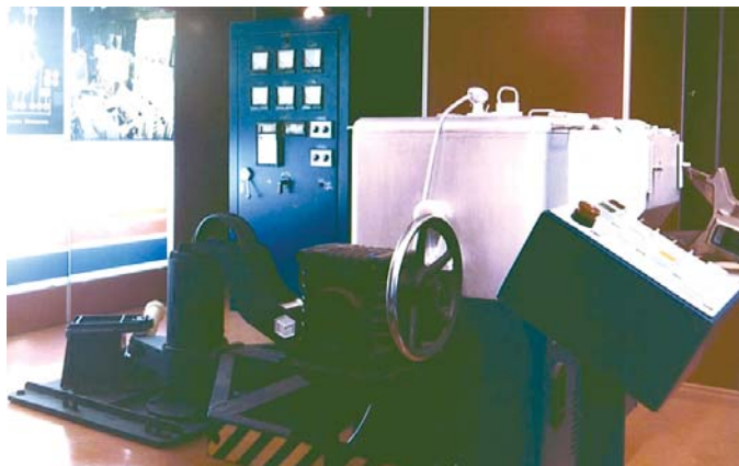
Magnetodynamic casting unit for smelting aluminum alloys
