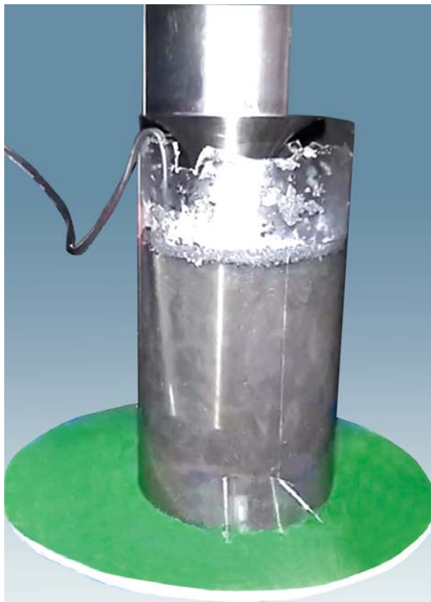
Processing of thermally expanded graphite in an ultrasonic disperser
