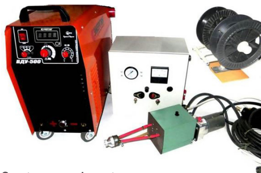
Stationary electric arc spray gun, control unit, cassette unit and power supply
