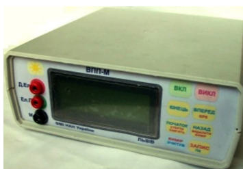
Device VPP for measuring of DC and AC electric voltages and polarization potential by a new method of extracting a resistance component
