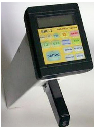
BVC-2: non-contact meter of currents and depths of pipe laying, search by three methods, control of insulation quality. The economy effect of 1.6 million €/year
