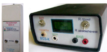
Devices VOZ for measuring of the resistance of ground and grounding in the area of EM hindrances
