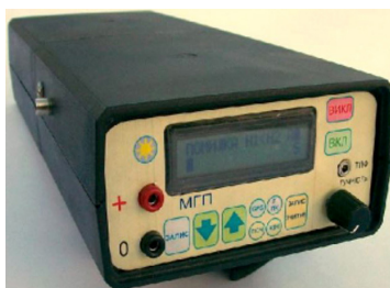
Device MGP to find and measure the depth of the pipeline and the electric potential
