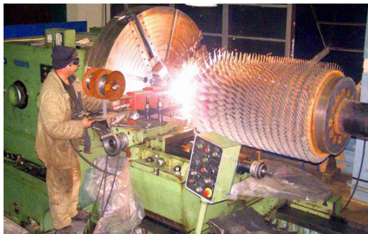
Restoration of basic necks turbine rotor compressor of gas compressor stations
