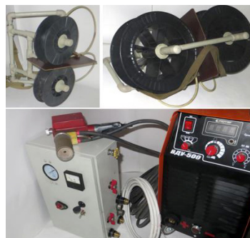
Mobile electric arc spray gun, control unit, cassette unit and power supply
