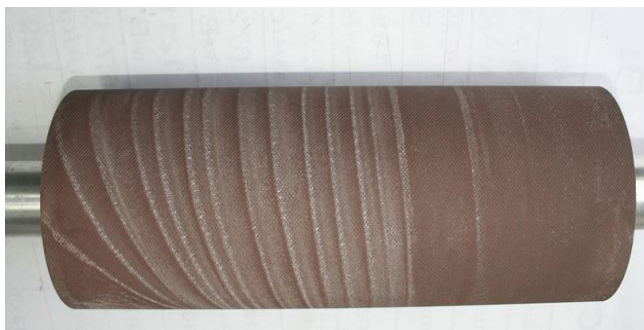
Wear-resistant coatings based on corundum synthesized on the surface of aluminum alloy leading and receiving cylinders on a printing machine Kosimax-Viva 340
