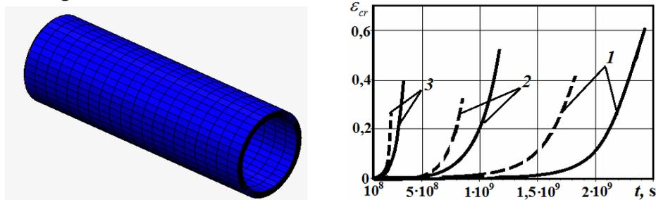
Fig. 1. Heat exchanger pipe fragment (a) and accumulation of creep strain over time in place of the highest strain energy on the outer wall of the pipe (solid lines), on the inner wall (dashed lines); without considering the environment (1), in 5% (2) and in 10 % solutions  $\text{MgCl}_2$  (3) (b)
