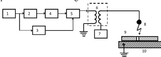
Fig. 1. Generalized scheme of PULSAR type holiday detector.
