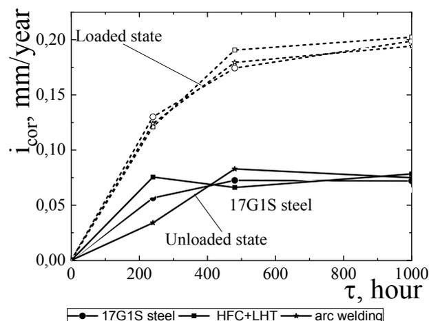
Fig. 1. Corrosion resistance of base metal of 17G1S steel and welded joints, received by high frequency welding (HFW) and arc welding (AW) after corrosion-mechanical investigations in unloaded and loaded states during 1000 hours of exposing to 3 % NaCl solution
