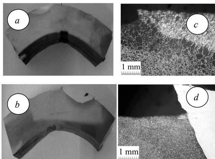
Fig. 1. Appearance of a fragment of a central part of welded joints of steel St3 (a, b) and microstructure of near-surface layers (c, d), with a ferrite deposited metal made by wire PPS AN-2 (a, c) and austenite deposited metal, made by wire of Ni strip (b, d), after study of resistance against corrosion cracking in a running flow during 250 h and bending up to initiation of the first crack
