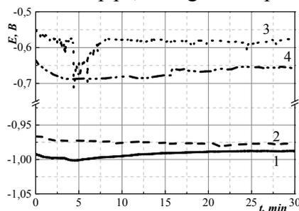
Fig. 1. Corrosion potential of galvanized pipe in the initial state (1-3) and after operation (4): 1) Zn on the outer surface; 2) Zn on the inner surface; 3) base metal; 4) Zn on the inner surface
