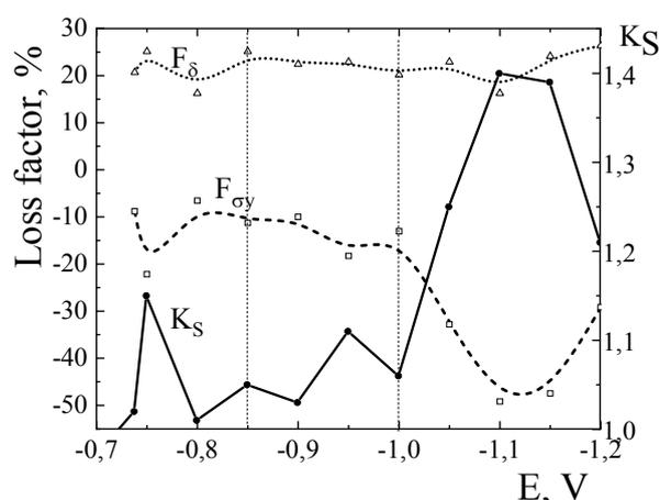
Fig. 1. Loss factors,  $F_{\delta}$  (elongation) and  $F_{\sigma_y}$  (yield stress), and sensitivity to SCC ( $K_S$ ) of 09G2S steel under cathodic polarization
