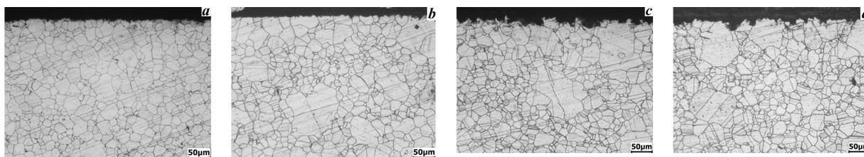
Fig. 1. The influence of the applied load on the change of the structure of the surface layer of austenitic steel Cr18Ni10Ti
