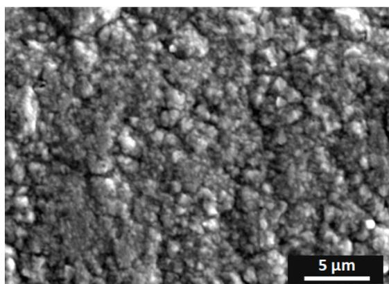
Fig. 1. SEM image of surface topography and morphology of Ni/Si<sub>3</sub>N<sub>4</sub>(15) composite coating
