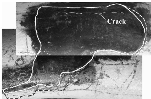
Fig. 1. Hydrogen induced delamination fracture of gas pipeline: delamination cracking under operation (solid line) and its extension after hydrostatic pressure testing (dotted line)
