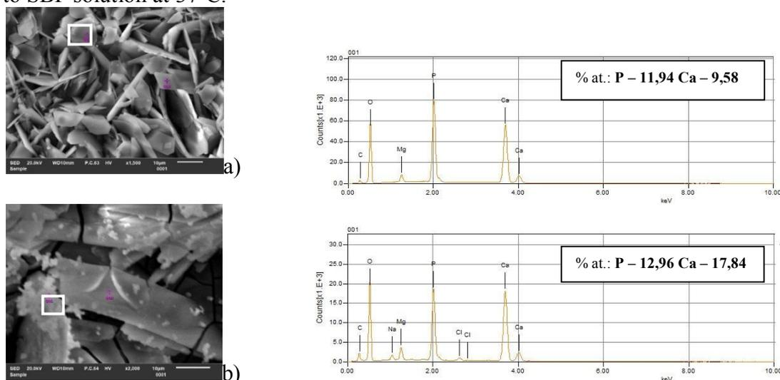
Fig. 1 SEM images and EDS analysis of calcium phosphate coating on RZ5 magnesium alloy before (a) and after (b) 9 days of immersion in SBF solution.
