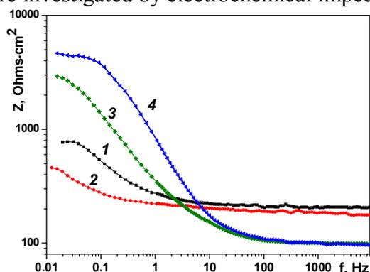
Fig. 1. Impedance dependence of carbon steel after a week of exposure at: 1) uninhibited 0,1 % NaCl; 2) 0,1 % NaCl+ 0,5g/l PST; 3) 0,1 % NaCl+ 2 g/l XG; 4) 0,1 % NaCl+2 g/l XG and 0,5g/l PST
