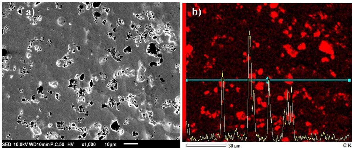
Fig. SEM image of surface topography (a) and carbon distribution (b) in a composite Ni/diamond coating
