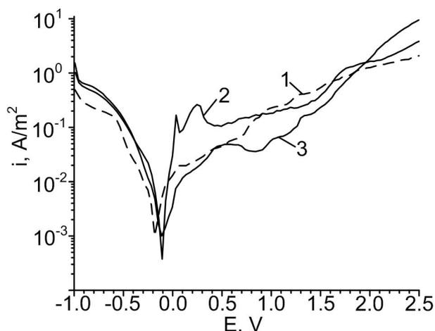
Fig. 1. Polarization curves of untreated (1), oxynitrided at 650°C (2) and 950°C (3) Ti64 alloy in 0.9% NaCl solution at 36°C
