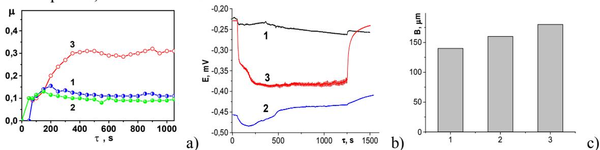
Fig. 1. Changes of friction factor (a), electrode potential on the friction surface (b), and friction track width (c) in solutions 3% NaCl (1), 3% NaCl + H<sub>2</sub>S (2), 3% NaCl + NH<sub>3</sub> (3)
