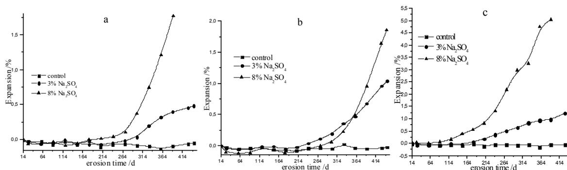
Fig. 1. The expansion of concrete under sulfate attack
