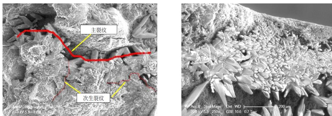
Fig. 2. SEM image of delayed ettringite
