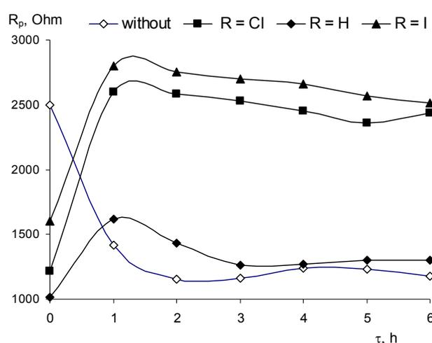
Fig. 2. Dependence between polarization resistance and sample soaking time in 0.2 M HCl solution (pH = 0.7)
