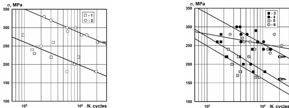
Fig.1 *S-N* curves of welded T-joints of 15KhSND steel as-welded (1) and treated by HFMI (2) in air; as-welded (3) and treated by HFMI (4) after corrosion tests; after pre-loading  $2 \cdot 10^6$  cycles and corrosion testing without HFMI treatment (5) and with further HFMI treatment (6)
