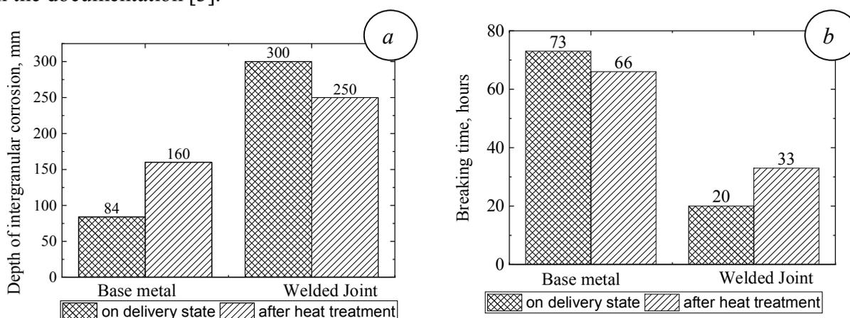
Fig.1. Influence of full heat treatment cycle on intergranular corrosion resistance (a) and resistance against corrosion-mechanical breaking (b)
