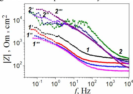
Fig. 1. Frequency dependencies of the impedance modulus of aluminum alloy samples in a non-inhibited solution of 0,1% NaCl (1) and with the addition of 2,5 g/l inhibitor TG (2) for temperatures: 1, 2 - 293 °K; 1', 2' - 313 °K; 1'', 2'' - 333 °K; 1''', 2''' - 353 °K.
