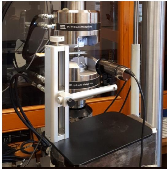
Fig. 1. Mode I fracture toughness test of the composite hybrid material
