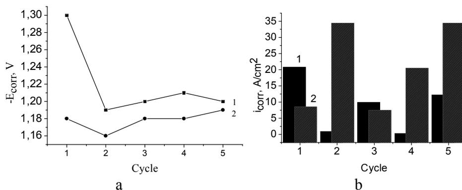
Fig. 2. a – Dependence of corrosion potential on the polarization cycle of AMAs: 1-  $\text{Al}_{87}\text{Y}_5\text{Ni}_8$ , 2-  $\text{Al}_{87}\text{Gd}_5\text{Ni}_8$ ; b – Dependence of corrosion currents on the polarization cycle of AMAs: 1-  $\text{Al}_{87}\text{Y}_5\text{Ni}_8$ , 2-  $\text{Al}_{87}\text{Gd}_5\text{Ni}_8$
