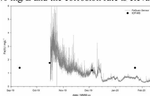
Fig. 2. Fe(II) determined by sensor values (line) and by ICP-MS (dots). Values are from a heating system in a high-rise building with hotel-business
