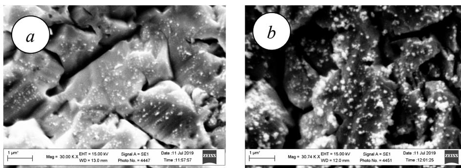
Fig. SEM images of Cu-porous/Ag-nano obtained by galvanic replacement of silver on dealloyed Cu-Zn system in AgNO<sub>3</sub> during 15 (a) and 45 s (b)
