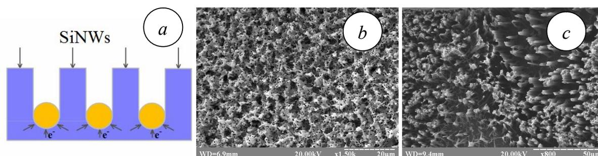
Fig. Scheme of contact metal activated silicon system Si/MNPs (a) and SEM images product of MACE – Si nanoporous (b) and SiNWs (c)
