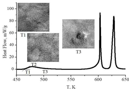
Fig. 1. DSC-curves of  $\text{Al}_{87}\text{Gd}_5\text{Ni}_8$  with a heating rate of 10 K/min.
