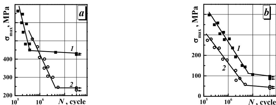
Fig. 1. Fatigue curves for the 34KhN3M in the initial state (1) and after operation during  $\sim 3 \times 10^5$  h in a rotor's disk of the steam turbine (2) which were obtained for testing in air (a) and in the model corrosive environment (b).
