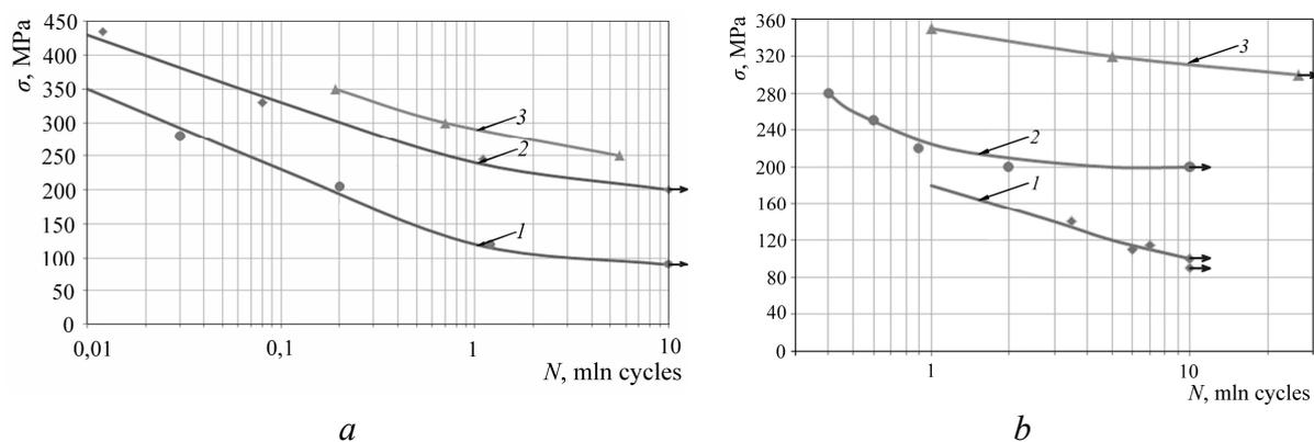
Fig. 1. Fatigue strength curves for the 20H2M (a) and 35XM (b) steels tested in air (1), in 3% NaCl solution (2) and the special technological environment (3).
