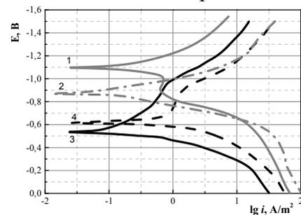
Fig. 2. Polarization curves on zinc coating (1-2) and steel (3-4) at different temperatures: 1) and 3) - 20 °C; 2) and 4) - 60 °C
