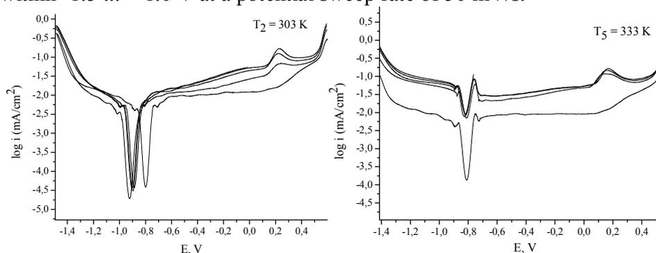
Fig. 1. Anodic polarization curves for  $\text{Co}_{72}\text{Si}_{11}\text{B}_{12}$  in 1 M KOH at different temperature.
