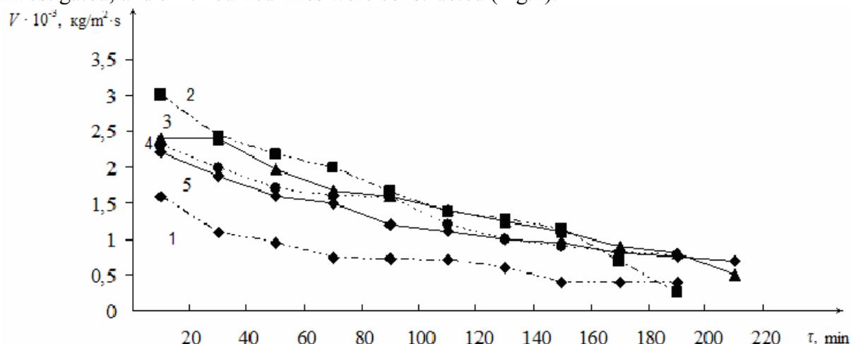
Fig. 1. Change in the etching rate of the alloy Cu98Be over time. In composition solutions mol/l: 1–0,5M FeCl<sub>3</sub>, 2–1,0M FeCl<sub>3</sub>, 3–0,5M FeCl<sub>3</sub> + 0,5M Fe(NO<sub>3</sub>)<sub>2</sub> + 0,5M HCl, 4–0,5M FeCl<sub>3</sub> + 0,5M Fe(NO<sub>3</sub>)<sub>2</sub> + 0,25M H<sub>2</sub>SO<sub>4</sub>, 5–0,5M FeCl<sub>3</sub> + 0,5M Fe(NO<sub>3</sub>)<sub>2</sub>
