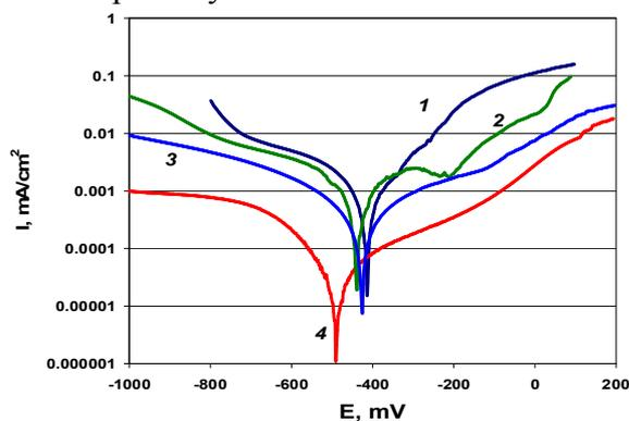
Fig. 1. Potentiodynamic polarization curves of D16T aluminium alloy after 24 hours exposure in acid rain solution: 1 – uninhibited, 2 – suspension with Ca-zeolite, 3 – suspension with phosphate Novinox PZ02, 4 – suspensions with complex pigment Ca-zeolite/zinc phosphate
