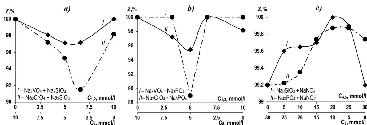
Fig. 1. Inhibitive efficiency vs concentration ratio of the binary mixture components.
