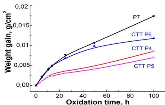
Fig. 1. The kinetics of oxidation of fuel cladding tubes from Zr-1%Nb alloy
