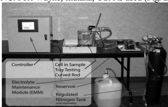
Fig. 2. Installation for determining the thickness of the oxide film
