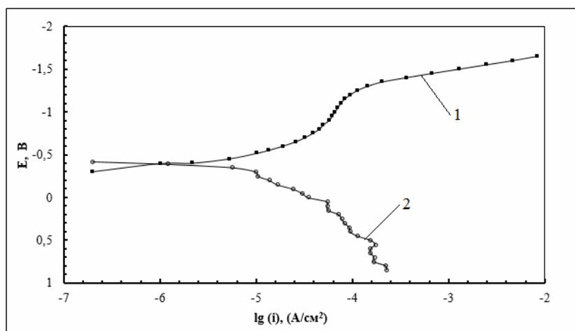
Fig. 1. Cathodic (1) and anodic (2) polarization curves of 65TiH<sub>2</sub>-30FeSiMn-5B<sub>4</sub>C composite in 3% NaCl solution
