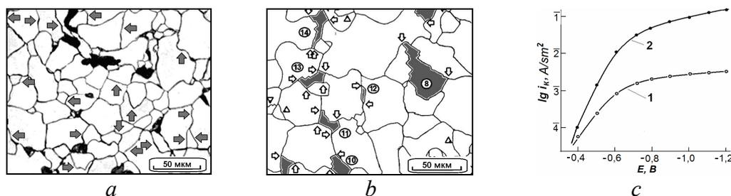
Fig. 1. Structure of 06Cr1-U steel tubes (a, b): a – SB  $\alpha$ - $\alpha$ ; b – SB  $\alpha$ - $\gamma$  (arrows); c – cathode polarization curves of 06Cr1-U steel (1) and 20 steel (2); 1N H<sub>2</sub>SO<sub>4</sub>+1.5g/l CS(NH<sub>2</sub>)<sub>2</sub>
