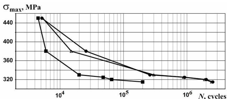
Fig. 1. Weller curve for basalt reinforcement:
