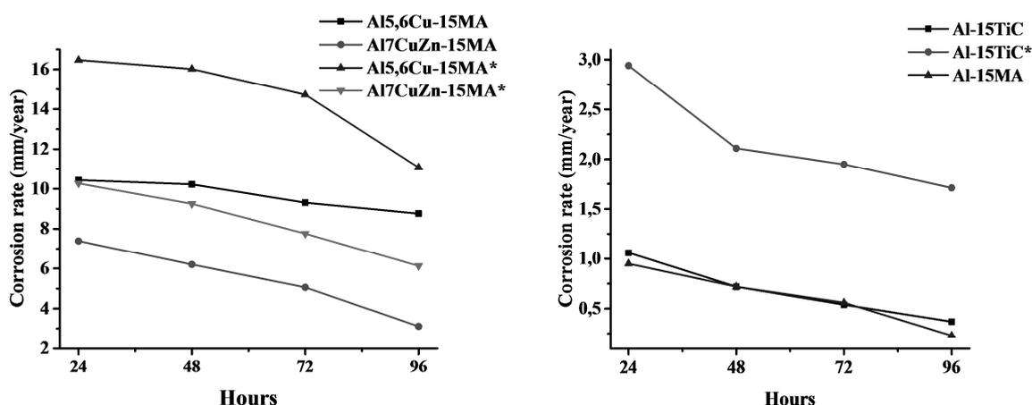
Fig. 1. Variation in the corrosion rate with the exposure duration in 3.5 wt.% NaCl and in 3.5 % NaCl + 10 % HCl (\*) solutions
