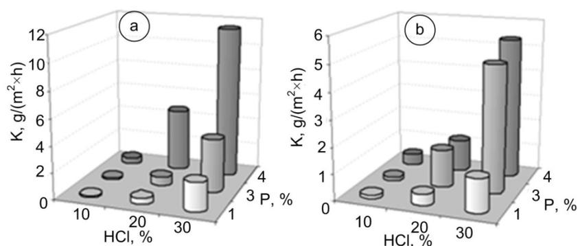
Fig. 1. Dependence of corrosion rate of sintered powder materials on their residual porosity in 10, 20 and 30% aqua solutions of hydrochloric acid: a – c.p. titanium; b – Ti-6Al-4V alloy
