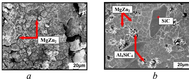
Fig. 1. The surface of unmodified (a) and SiC laser-modified (b) alloy 7075 particles after corrosion of a 3% NaCl solution for 192 h
