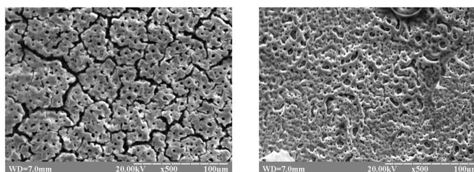
Fig. 1. Ti-Zr PEO treated surface without (left image) and with (right image) chitosan coating after incubation in H<sub>2</sub>SO<sub>4</sub>/NaCl solution
