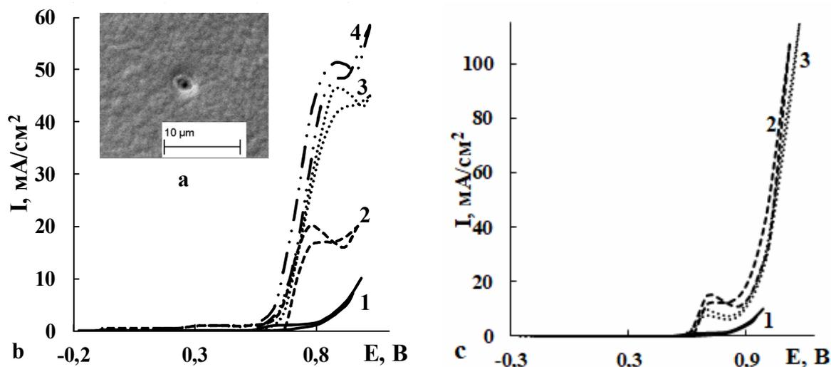
Fig. 1. a) SEM micrograph and voltammograms of the Ni-Cu coatings in 1M NaOH in the absence (1) and presence of b) 0,3M (2), 1M (3), 2M  $\text{CH}_3\text{OH}$  (4); c) 1M (2), 2M  $\text{C}_2\text{H}_5\text{OH}$  (3)
