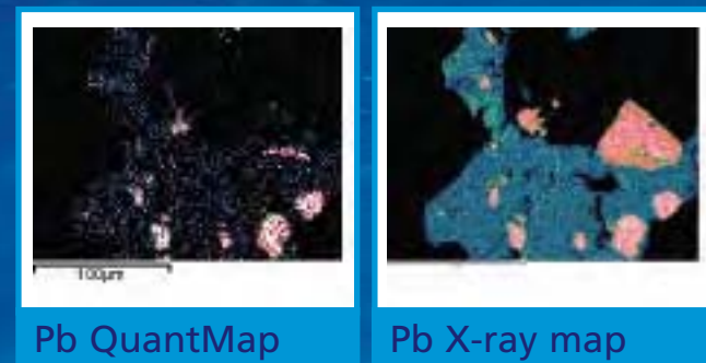
The example shows Pb X-ray map and a Pb Quantmap for the same area. The sample also contains significant levels of S, which overlaps with the Pb M line. The Pb X-ray map is showing the distribution of both Pb and S, whereas the Pb Quantmap shows the correct distribution of Pb.
